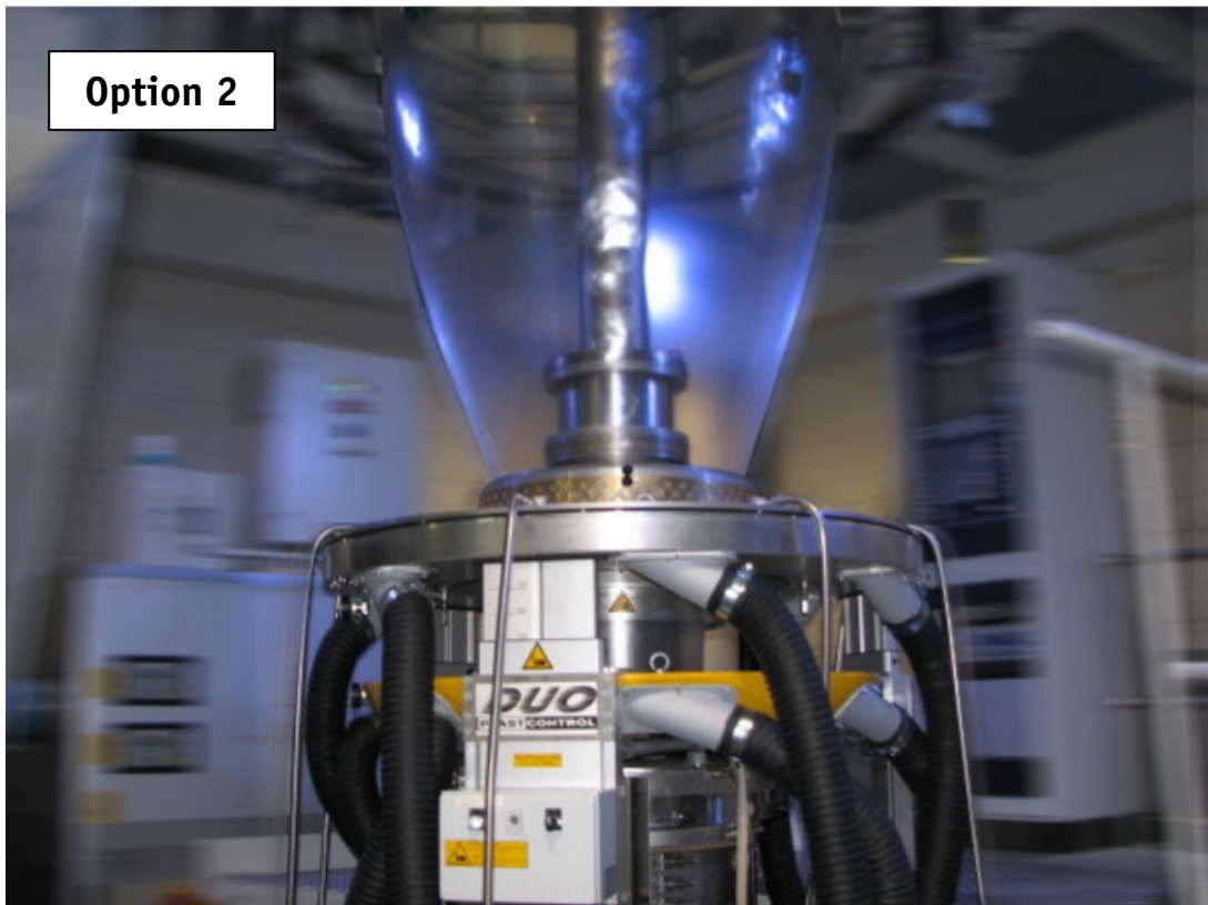
Double stack air ring DU0 option 2 with 64 Thermocouples for profile control
