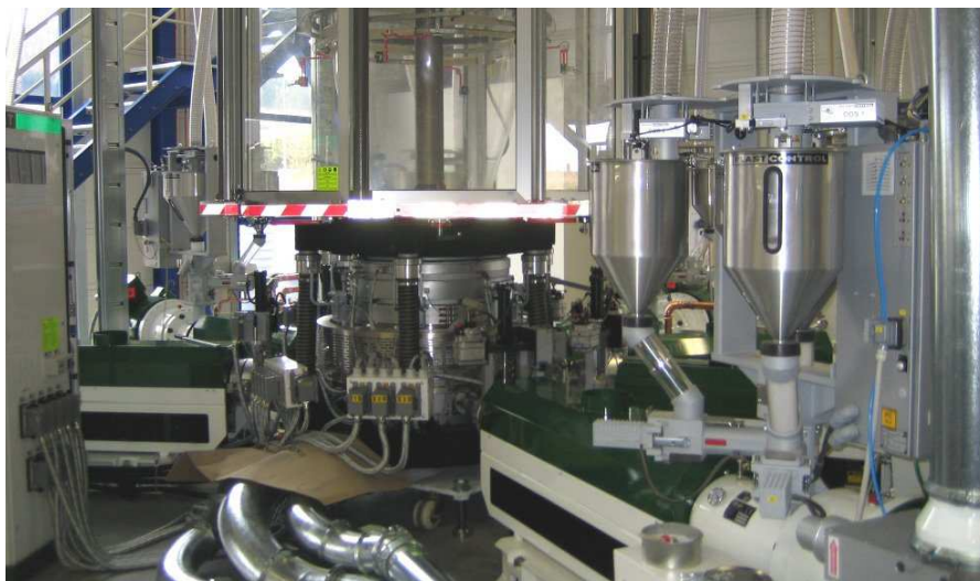
7-layer Co-Extrusion line with gravimetric dosing units
